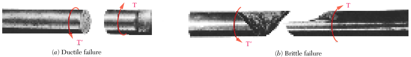
Photo 3.2 Shear failure of shaft subject to torque.
