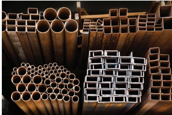
Photo 6.3 Box beams and tubes.
