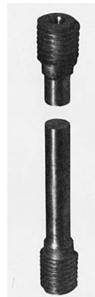
Photo 2.5 Tested specimen of a brittle material.
