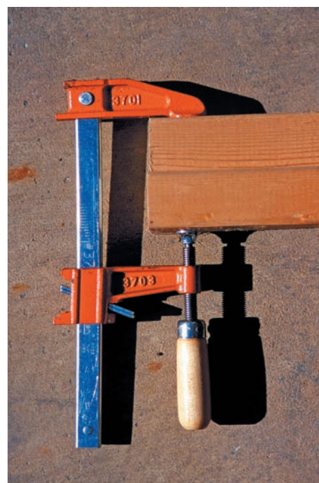
Photo 4.2 Clamp used to glue lumber pieces together.
