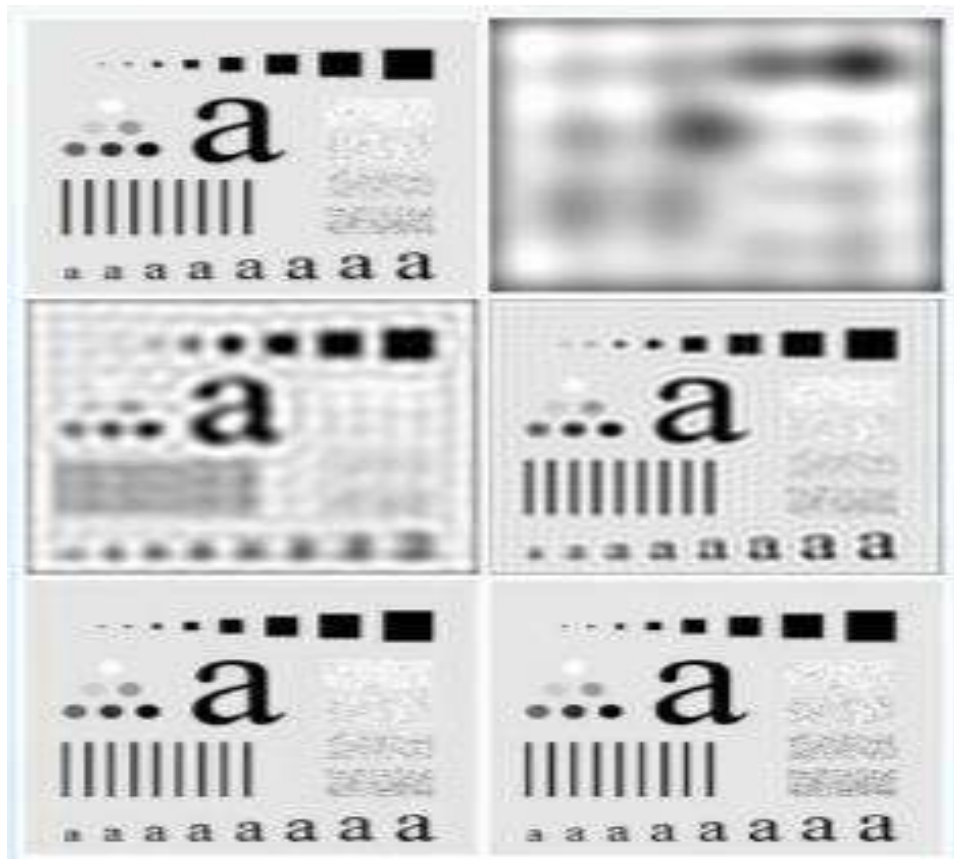
Fig: (a) original image, (b)-(f) Results of filtering using ILPFs with cutoff frequencies set at radii values 10, 30, 60, 160 and 460, as shown in figure. The power removed by these filters was 13, 6.9, 4.3, 2.2 and 0.8% of the total, respectively.
