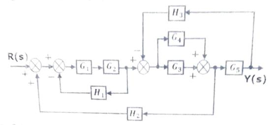
e) Obtain the overall transfer function C / R of the following system by using Mason's gain formula
