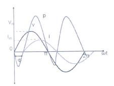
As seen from the power waveform, the instantaneous power is alternately positive and negative. When the power is positive, the power flows from the source to the load and when the power in negative, the power flows from the load to the source. The positive power is not equal to the negative power and hence the average power in the circuit is not equal to zero.
