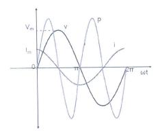
As seen from the power waveform, the instantaneous power is alternately positive and negative. When the power is positive, the power flows from the source to the capacitor and when the power in negative, the power flows from the capacitor to the source. The positive power is equal to the negative power and hence the average power in the circuit is equal to zero. The power just flows between the source and the capacitor, but the capacitor does not consume any power.
