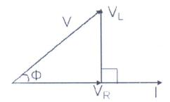
The current I is taken as the reference phasor. The voltage  $V_R$  is in phase with I and the voltage  $V_L$  leads the current by 90°. The resultant voltage V can be drawn as shown in the figure. From the phasor diagram we observe that the voltage leads the current by an angle  $\Phi$  or in other words the current lags behind the voltage by an angle  $\Phi$ .
