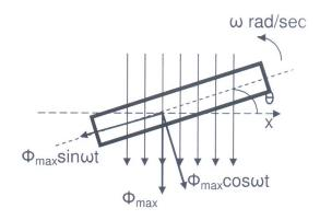
The component of flux acting along the plane of the coil does not induce any flux in the coil. Only the component acting perpendicular to the plane of the coil ie  $\Phi_{max}$ cos $\omega$ t induces an emf in the coil.
