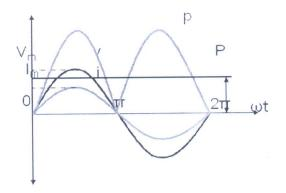
As seen from the waveform, the instantaneous power is always positive meaning that the power always flows from the source to the load.
