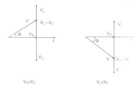
From the phasor diagram we observe that when  $V_L > V_C$ , the voltage leads the current by an angle  $\Phi$  or in other words the current lags behind the voltage by an angle  $\Phi$ . When  $V_L < V_C$ , the voltage lags behind the current by an angle  $\Phi$  or in other words the current leads the voltage by an angle  $\Phi$ .
