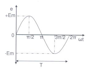
An alternating quantity changes continuously in magnitude and alternates in direction at regular intervals of time. Important terms associated with an alternating quantity are defined below.
