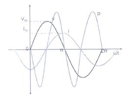
As seen from the power waveform, the instantaneous power is alternately positive and negative. When the power is positive, the power flows from the source to the inductor and when the power in negative, the power flows from the inductor to the source. The positive power is equal to the negative power and hence the average power in the circuit is equal to zero. The power just flows between the source and the inductor, but the inductor does not consume any power.
