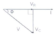
The current I is taken as the reference phasor. The voltage  $V_R$  is in phase with I and the voltage  $V_C$  lags behind the current by  $90^{\circ}$ . The resultant voltage V can be drawn as shown in the figure. From the phasor diagram we observe that the voltage lags behind the current by an angle  $\Phi$  or in other words the current leads the voltage by an angle  $\Phi$ .
