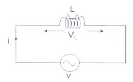
Consider an AC circuit with a pure inductance L as shown in the figure. The alternating voltage v is given by  $v = V_m \sin \omega t \tag{1}$
