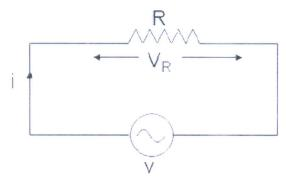
Consider an AC circuit with a pure resistance R as shown in the figure. The alternating voltage v is given by  $v = V_m \sin \omega t$
