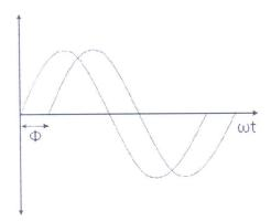
When two alternating quantities of the same frequency have different zero points, they are said to have a phase difference. The angle between the zero points is the angle of phase difference.
