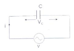
The current flowing in the circuit is i. The voltage across the capacitor is given as  $V_C$  which is the same as v.
