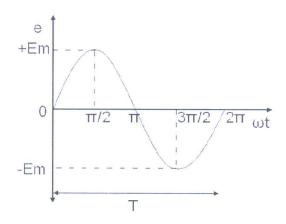
Phase is defined as the fractional part of time period or cycle through which the quantity has advanced from the selected zero position of reference
