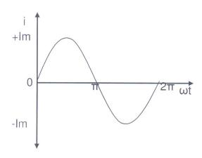
$i = I_m \sin \omega t$   $I_{av} = \frac{1}{\pi} \int_{0}^{\pi} id(\omega t)$   $I_{av} = \frac{1}{\pi} \int_{0}^{\pi} I_m \sin \omega t d(\omega t)$
