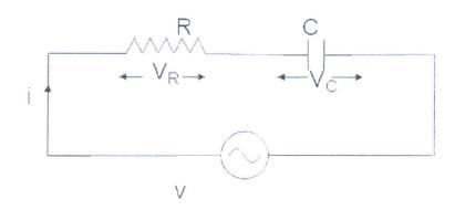
Consider an AC circuit with a resistance R and a capacitance C connected in series as shown in the figure. The alternating voltage v is given by
