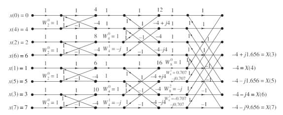
**Figure 7.38** Computation of 8–point DF $\dagger$  of x(n) by radix–2, DI $\dagger$  FF $\dagger$ .
