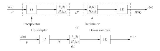
Figure 5.19 Cascading of sample rate converters.
