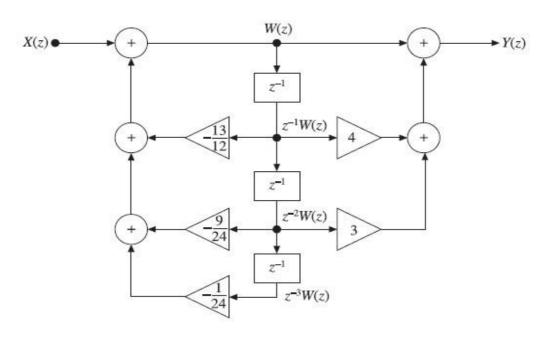
**EXAMPLE 1.2.4** Find the direct form-I and direct form-II realizations of a discrete-time system represented by the transfer function
