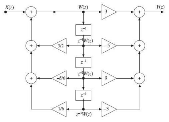
Figure 1.2.14 Realization of IIR system through direct form-II
