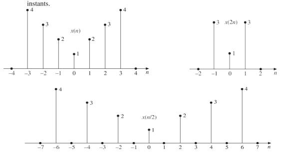
**Figure 1.16** Discrete—time scaling (a) Plot of x(n) (b) Plot of x(2n) (c) Plot of x(n/2) Time scaling is very useful when data is to be fed at some rate and is to be taken out at a different rate.
