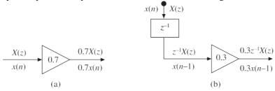
**Figure 1.2.2** BFock diagram representation of (a) 0.7X(z) and (b)  $0.3z^{-1}X(z)$ .
