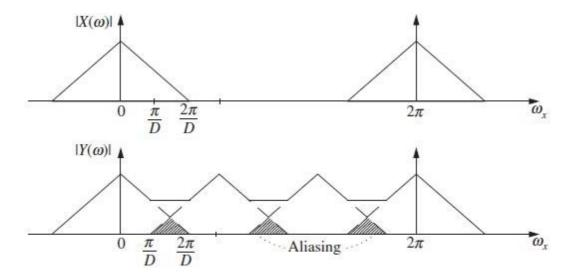
Figure 5.5 (a) Input spectrum, (b) aliased output spectrum.
