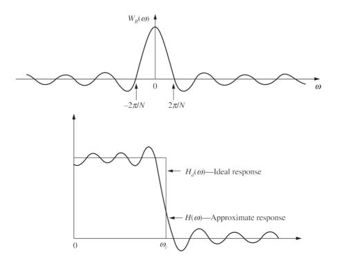
**Figure 3** (a) Rectangular window sequence, (b) Magnitude response of rectangular window, (c) Magnitude response of Now-pass filter approximated using rectangular window.
