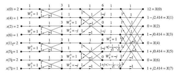
**Figure 7.33** Computation of 8–point DF† of x(n) by radix–2 DIF FF† aFgorithm.
