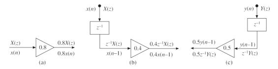
Figure 1.2.4 BFock diagram representation of (a) 0.8X(z) (b)  $0.4z^{-1}X(z)$  and (c)  $0.5z^{-1}Y(z)$ .
