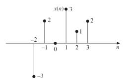
Figure 1.2 Graphical representation of discrete-time signal
