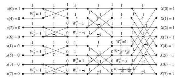
**Solution:** (a) 8-point DFT by Radix-2 DIT FFT algorithm
