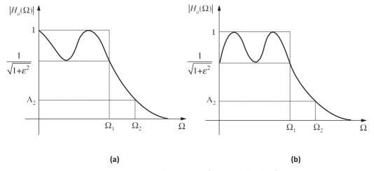
Figure 6 Magnitude response of type-I Chebyshev filter.
