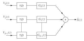
Figure 5.26 Synthesis filter bank.
