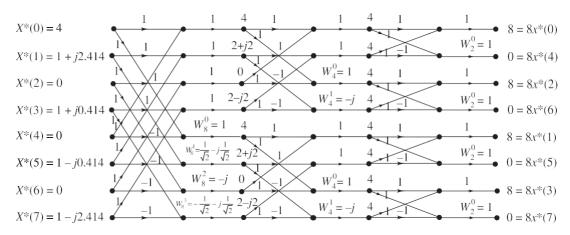
**Figure 7.42** Computation of 8–point DF† of  $X^*(k)$  by radix–2 DIF FF†.
