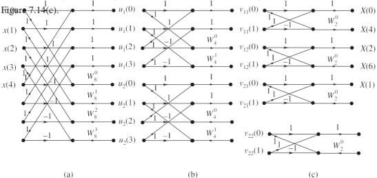
$\textbf{Figure 7.14} \quad \text{(a)--(c) $\dagger$ he first, second and third stages of computation of $8$-point DF$ $\dagger$ by Radix-2 DIF FF$$\dagger$. }$
