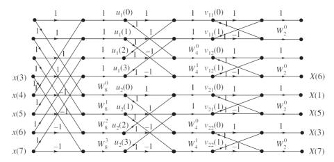
Figure 7.13 SignaF fFow graph or butterfFy diagram for the 8-point radix-2 DIF FF† aFgorithm.
