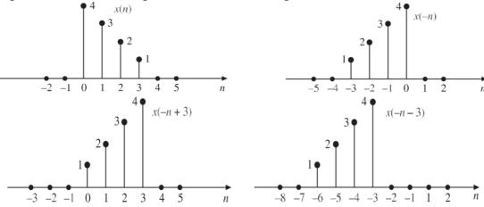
**Figure 1.11** (a) Original signal x(n) (b) Time reversed signal x(-n) (c) Time reversed and delayed signal x(-n+3) (d) Time reversed and advanced signal x(-n-3).
