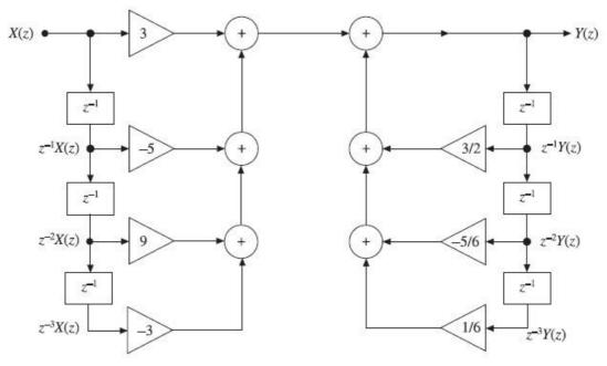
Figure 1.2.13 Realization of IIR system through direct form-I
