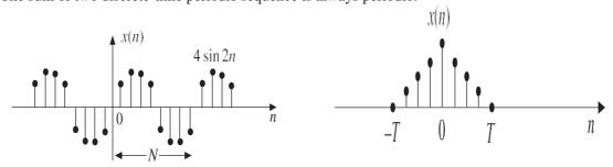
some examples of discrete-time periodic/non-periodic signals are shown in Figure 1.19. Figure 1.19 Example of discrete-time: (a) Periodic and (b) Non-periodic signals
