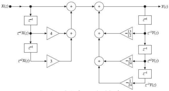
Figure 1.2.11 Realization of IIR system through direct form—I
