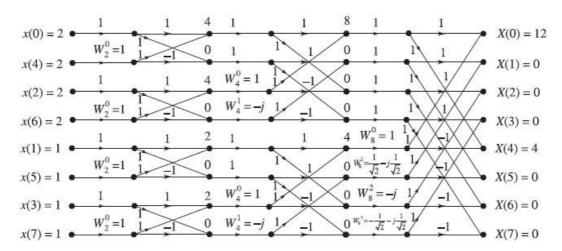
**Figure 7.35** Computation of 8–point DF† of x(n) by radix–2, DI† FF†.
