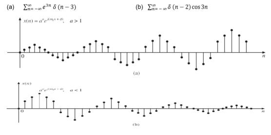
Figure 1.9 complex exponential sequence  $x(n) = a^n e^n (\omega_0 n + \emptyset)$  for (a)a > 1 (b) a < 1.
