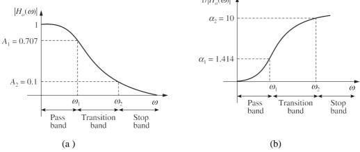
**Figure 3** Magnitude response of low–pass filter (a) Gain vs  $\omega$  and (b) Attenuation vs  $\omega$ . Let  $\omega_1 = Passband$  frequency in rad/s.  $\omega_2 = Stopband$  frequency in rad/s.
