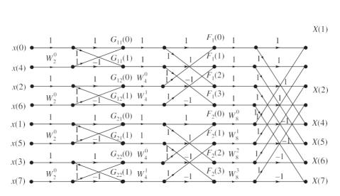
Figure 7.8 †he signal flow graph or butterfly diagram for 8-point radix-2 DIT FFT.
