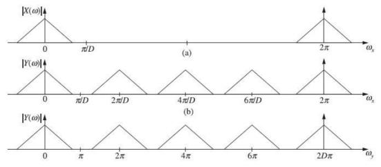
Figure 5.4 Spectrum of (a) input, (b) output, and (c) normalized output.
