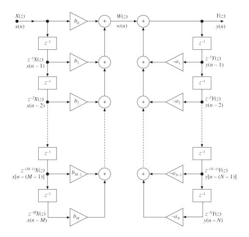
Figure 1.2.6 Direct form—I structure.
