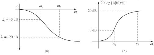
Figure 4 Magnitude response of low–pass filter (a) dB–Gain vs  $\,\omega$  and (b) dB–attenuation vs  $\,\omega$  .
