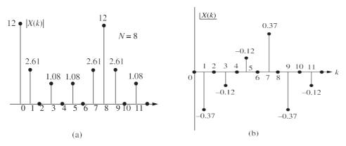
Figure 7.34 (a) Magnitude spectrum, (b) Phase spectrum.
