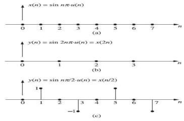
**Figure 5.12** Plots of (a)  $x(n) = \sin n \ u(n)$ , (b)  $y(n) = \sin 2n \ u(n)$  and (c)  $y(n) = \sin (n/2)u(n)$ .
