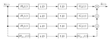
**Figure 5.27** Sub–band coding filter bank. □
