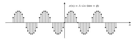
Figure 1.7 Discrete-time sinusoidal signal
