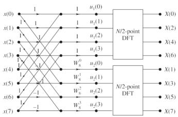
**Figure 7.9** FFow graph of the DIF decomposition of an N-point DF† computation into two N/2-point DF† computations N = 8.
