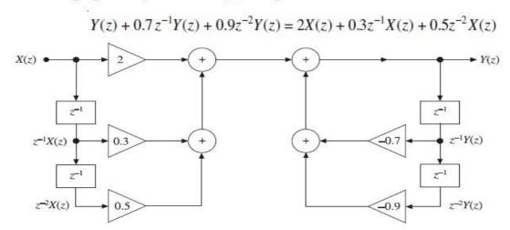
Figure 1.2.15 Realization of IIR system through direct form-I
