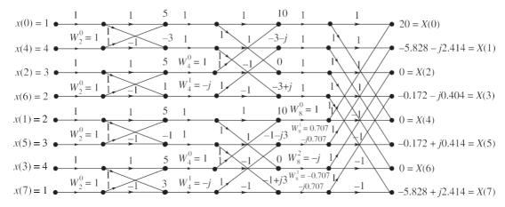
**Figure 7.37** Computation of 8–point DF† of x(n) by radix–2, DI† FF†.
