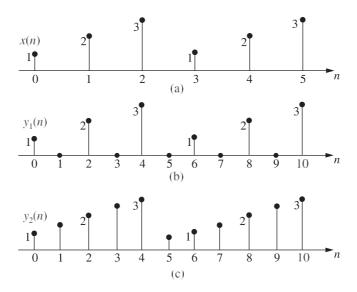
**Figure 5.7** (a) Input signal x(n), (b) Output of 2 fold up sampler  $y_f(n) = x(n/2)$ , (c) Output of interpolator  $y_2(n) = x(n/2)$ .
