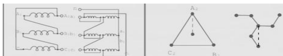
Fig5.19.Dz6 connection and phasor diagram
