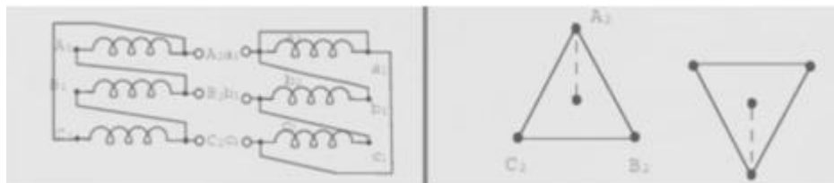
Fig5.11 Dd6 connection and phasor diagram
