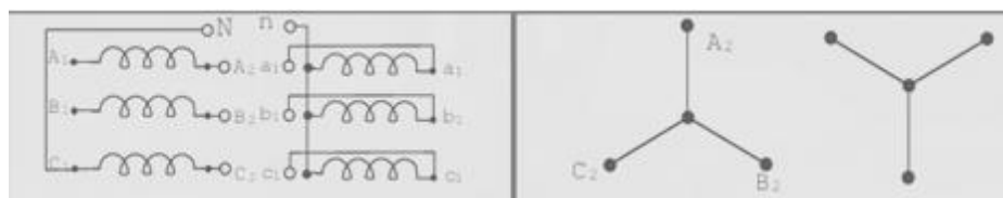
Fig 4.13. Yy6 connection and phasor diagram
