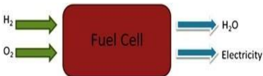
General concept of a H_2 - O_2 fuel cell
