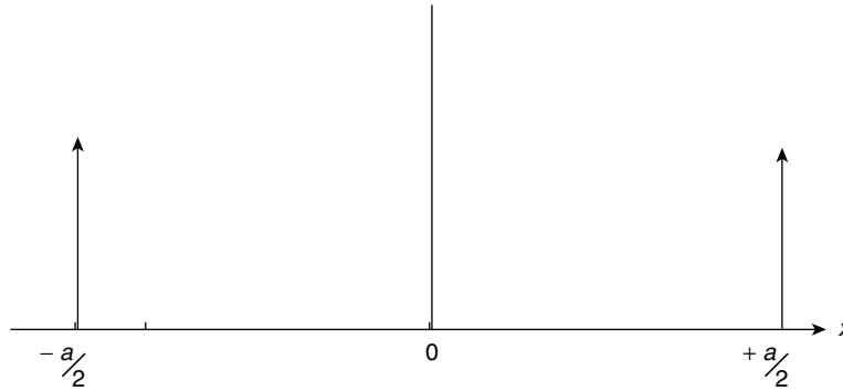
Figure 10.14 The Fourier transform of two Dirac \delta functions located at x = \pm a/2 is 2 \cos ka/2
