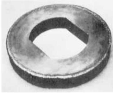
FIGURE 1.38 Mild-steel die on the edge of which tool steel has been deposited by means of tool-steel electrode.
