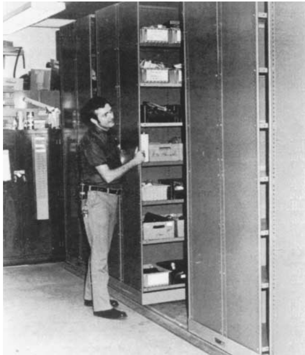
FIGURE 8.8 Movable bins, equipped with rollers on floor tracks.
