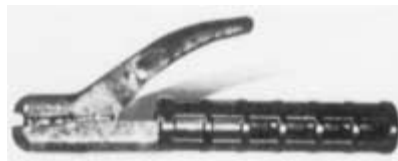
FIGURE 1.50 Fully insulated electrode holder designed especially for cool operation.
