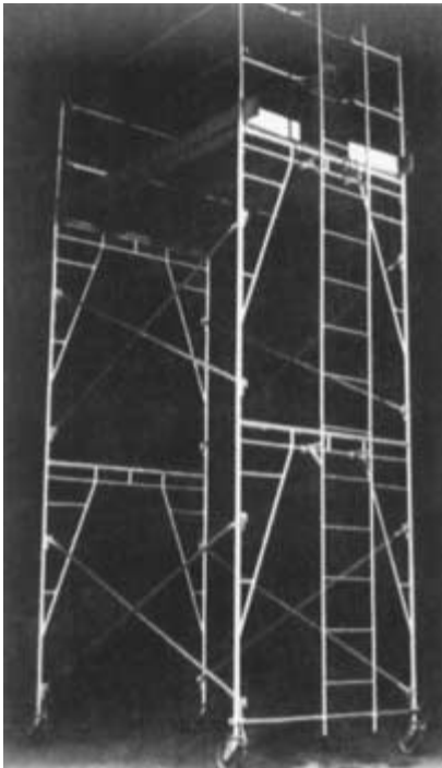
FIGURE 10.5 Sectional rolling scaffold. Steel frames are 5 ft wide and joined by pivoted diagonal braces of lengths from 4 to 10 ft. A “hook-on” type of access ladder is used incorporating a 3-ft-high grabrail at top, guarded by steel wire rope with snap hooks. The complete lift of the ladder is set back 7½ in. from the scaffold frames.
