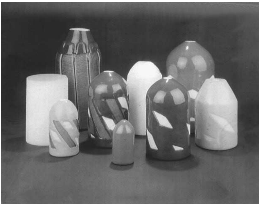
FIGURE 2.8 Specialized foam pigs are available for almost every pipeline cleaning requirement, from light cleanings, wiping, and drying (squeegeeing), to heavy buildup removal and scraping. Pigs can be used in lines of less than 2 in. diameter to 144 in. (12 ft) diameter. These various pigs have a concave base and conical head design to increase speed and effectiveness, and the spiral/crisscross bands of abrasive material create a patented rotating motion, further enhancing cleaning. (Courtesy of Girard Industries, Inc., Houston, Tex.)
