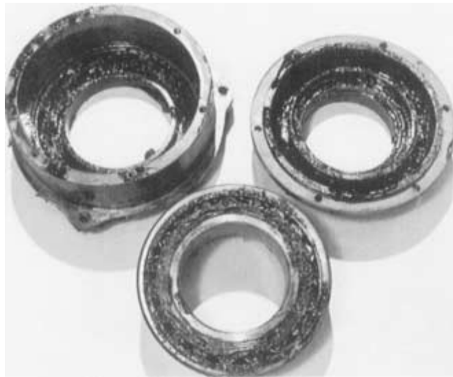
FIGURE 1.9 Excessive lubrication can cause overheating of bearings and contamination within the motor.
