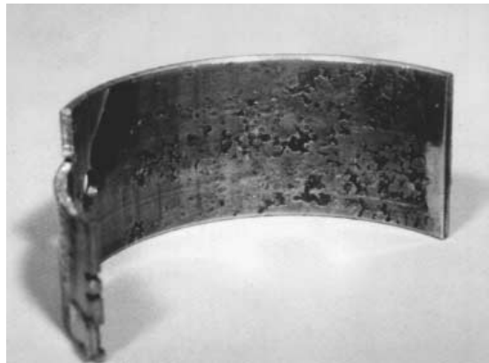
FIGURE 1.10 Fatigue of bearing lining.
