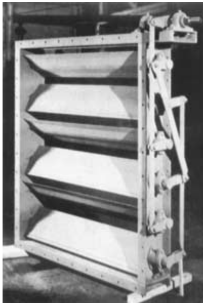
FIGURE 7.12 Outlet damper with streamlined blades and linkage arranged to move adjacent blades in opposite directions for even throttling.
