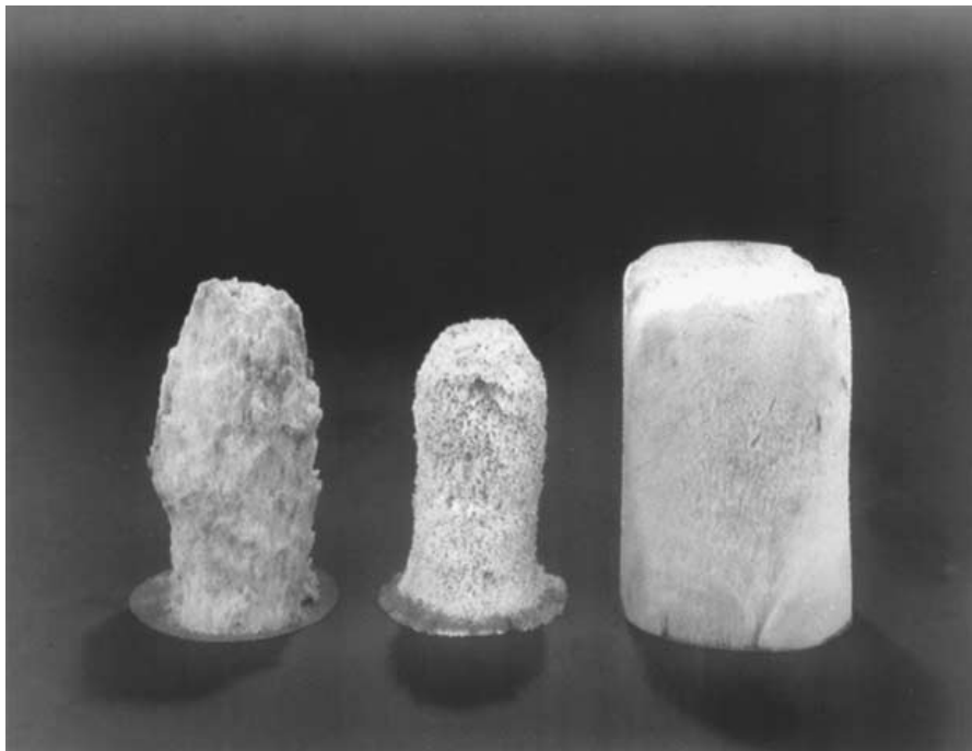
FIGURE 2.5 Pipeline plugs showing deterioration.
