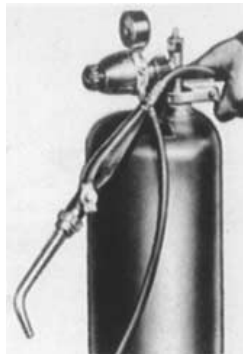
FIGURE 2.2 Connecting a typical air-acetylene outfit. The standard type of portable outfit is shown. Smaller tanks also are available.
