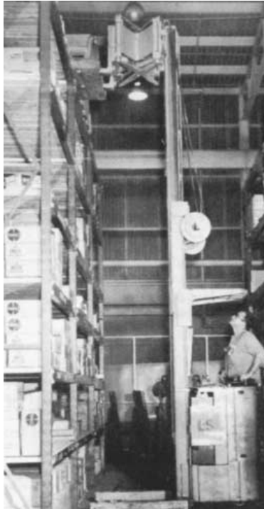
FIGURE 8.4 Fork truck used for high vertical lifts of palletized material.
