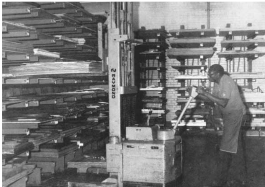
FIGURE 8.5 Small forklift truck used for handling metal plate and similar material.
