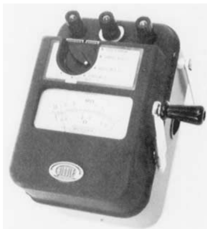
FIGURE 2.26 Portable megger. (James G. Biddle Company.)
