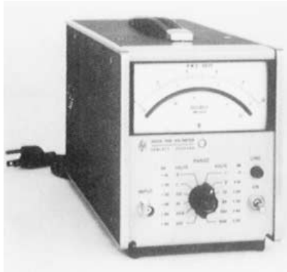
FIGURE 2.18 Electronic-type true rms meter. ( Hewlett-Packard. )
