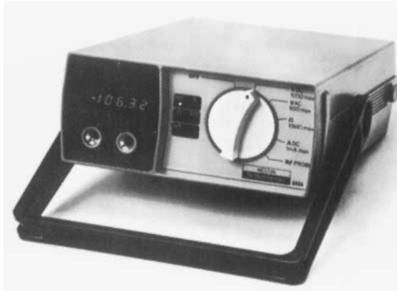
FIGURE 2.6 Four-digit autoranging DMM. (Weston Instruments, Inc.)
