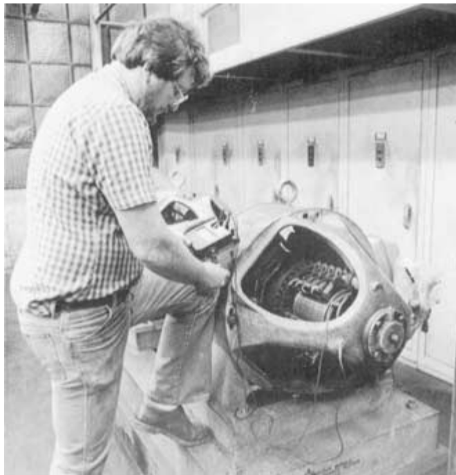
FIGURE 1.19 Megger testing insulation on a d-c motor.
