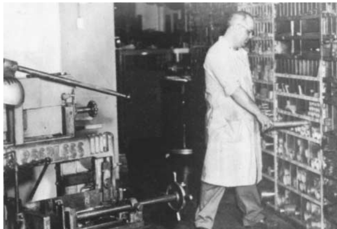
FIGURE 8.3 Power hacksaw in metals storeroom, used with other cutting equipment to issue requested lengths and sizes.
