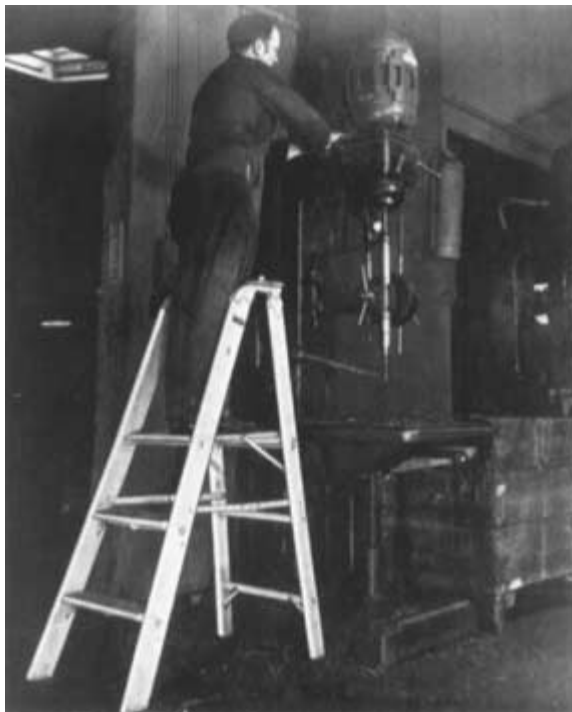
FIGURE 10.2 Platform stepladder. Preferred because it permits worker to have both hands free.
