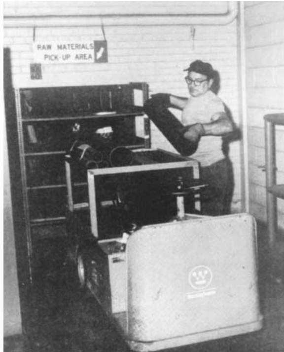
FIGURE 8.2 Small delivery truck suitable for use either in plant aisles or between buildings.
