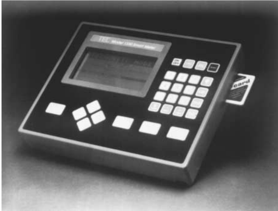
FIGURE 3.20 Microprocessor-based vibration analyzer.
