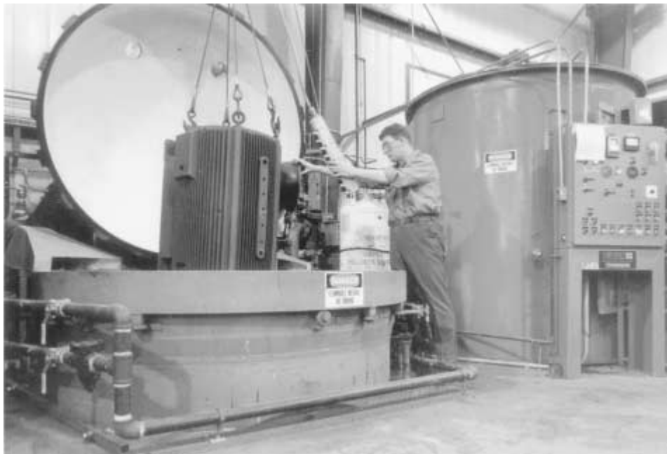
FIGURE 1.6 A-c stator being lowered into VPI tank.
