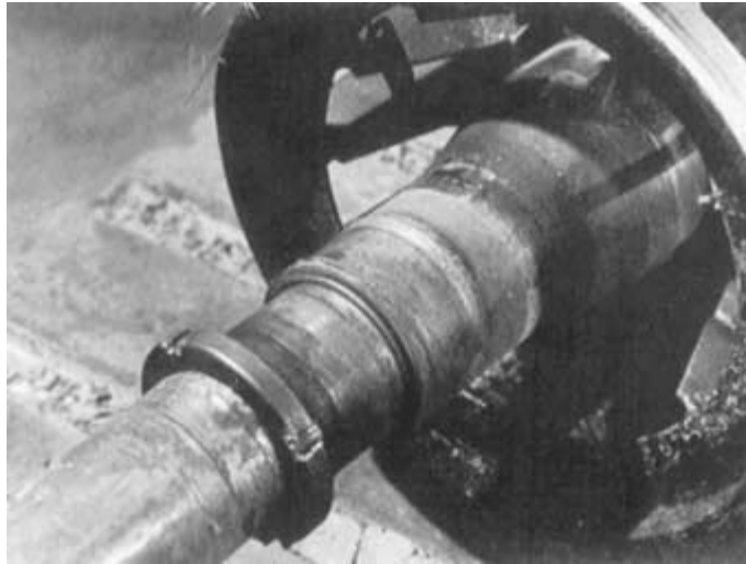
FIGURE 1.12 The shaft bearing seat has become scored due to the bearing overheating in Fig. 1.11.
