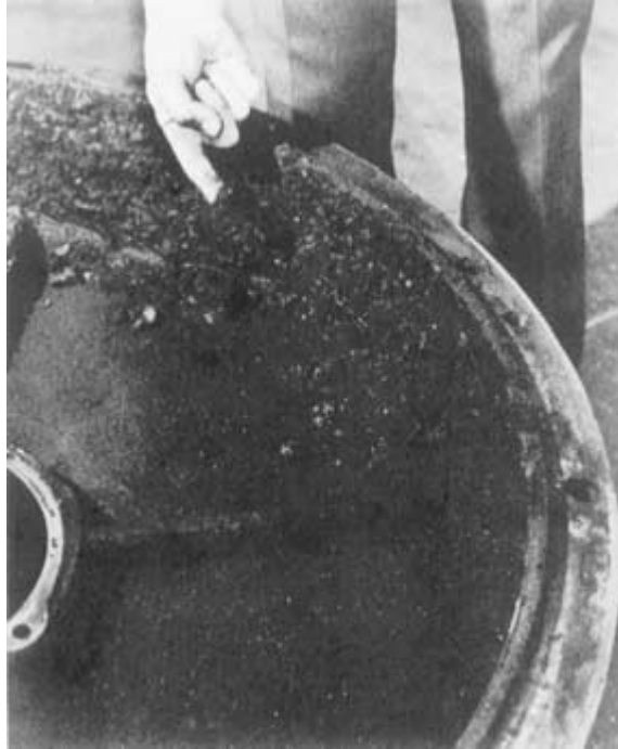
FIGURE 1.10 Dirt and grease buildup as a result of overlubrication.
